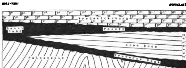
FIG. 1688. — Ideal section showing the relationships of the Trinity and Fredericksburg formations of the Texas Comanchean. The basal sandstone (in black) rises in the scale with the advance of the sea; the Paluxy sandstone (also in black) represents a combined sandstone of emergence and submergence. (Original.)
